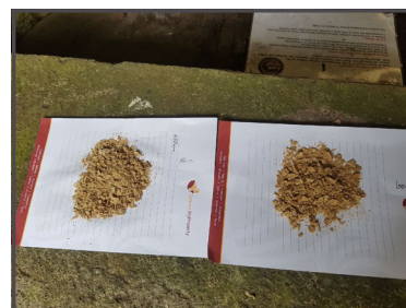
The left post was replaced and the other posts tested. Quality test samples from forensic investigation of the post timbers.
