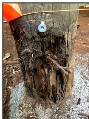
The left post was replaced and the other posts tested. Quality test samples from forensic investigation of the post timbers.
